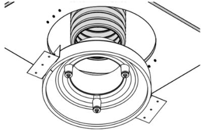
**Step 4.** Install the ceiling valve into the hole in the ceiling. The mounting brackets must be supported with the back side of the plasterboard. Align the mark on the ceiling valve with the centre of the hole in the middle.
