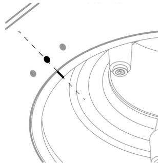
**Step 5.** Secure the ceiling valve with screws. Install the front panel fixed with magnet holders.
