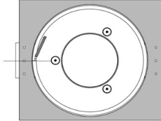
**Step 2.** Align the template with the ceiling and mark up the places to install the ceiling valve and make holes for mounting. Make a hole in the plasterboard. Cut the chamfer at a 45° angle up to 1/3 plasterboard thickness.
