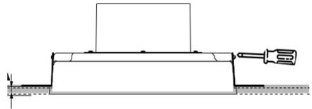
Before starting the installation, secure the mounting brackets in pre-made holes on the ceiling valve's casing. Adjust the position of the mounting brackets based on the ceiling thickness.
